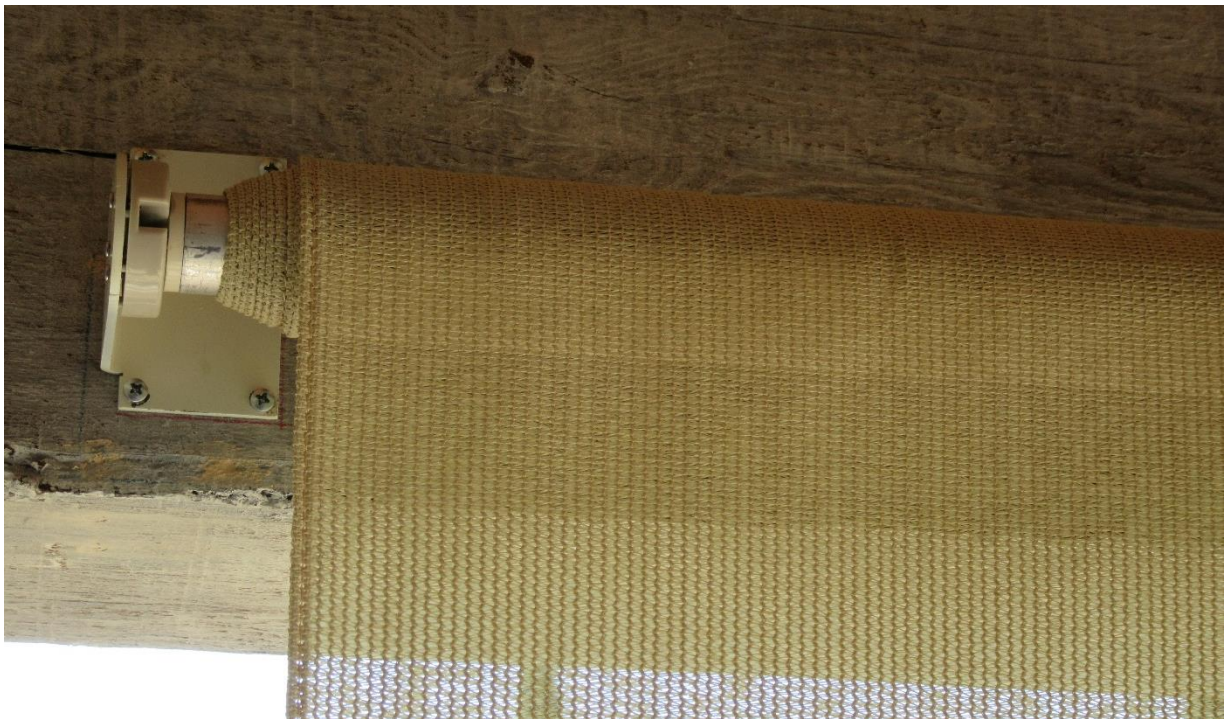
Figure 22 - Telescoping at Idler End of Shade
