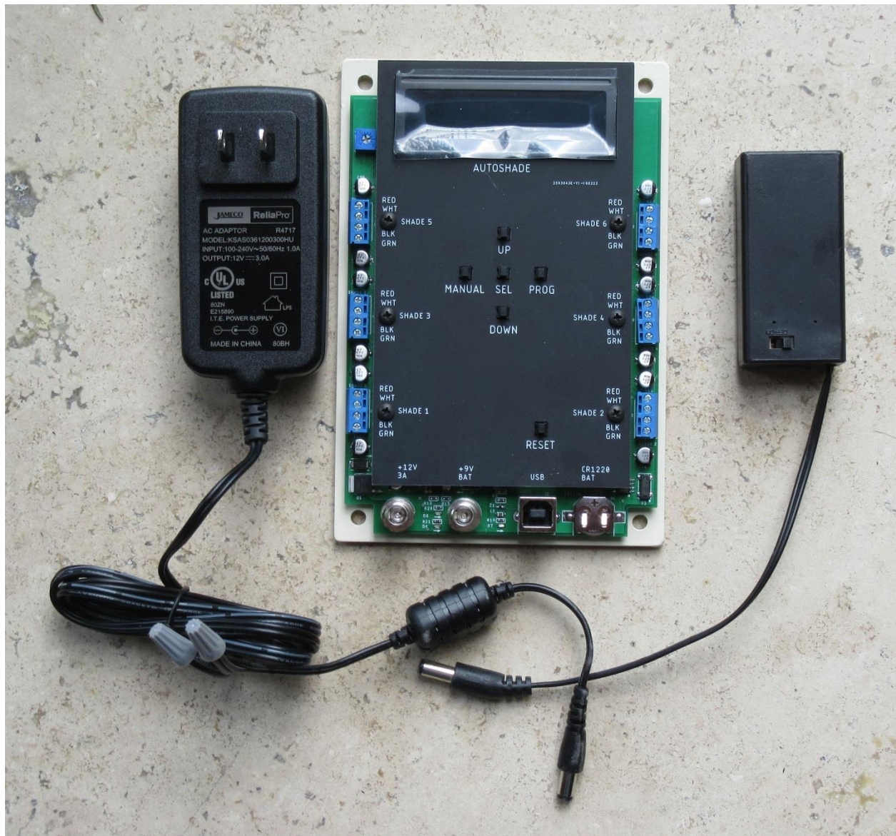
Figure 2 - Autoshade Controller Assembly
